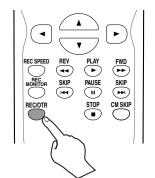
Rrecording times appear on the TV screen (30 minutes to 4 hours). Recording will start.
